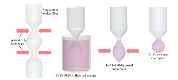
Fig. S1. Fabrication process of an Er-Yb co-doped microsphere cavity.
