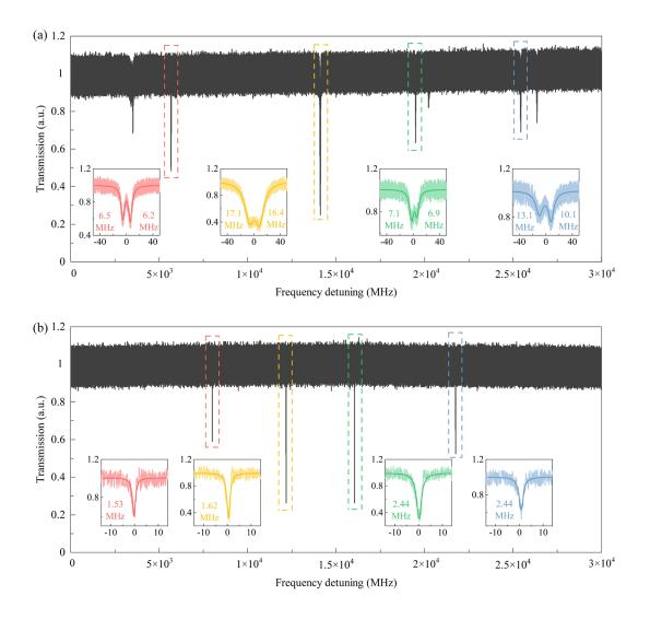
**Fig. S3.** Typical transmission spectra around 1620 nm of the Er-Yb co-doped microspheres (a) without and (b) with the assistance of PMMA. Insets: Zoom-in transmission spectra, where the fitted linewidths corresponding to the four resonance modes are exhibited.
