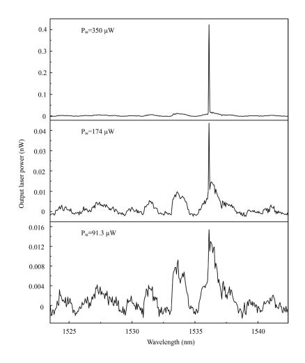
Fig. S9. Detailed evolution of the Er-ion downshifting spectra as the pump power increases.
