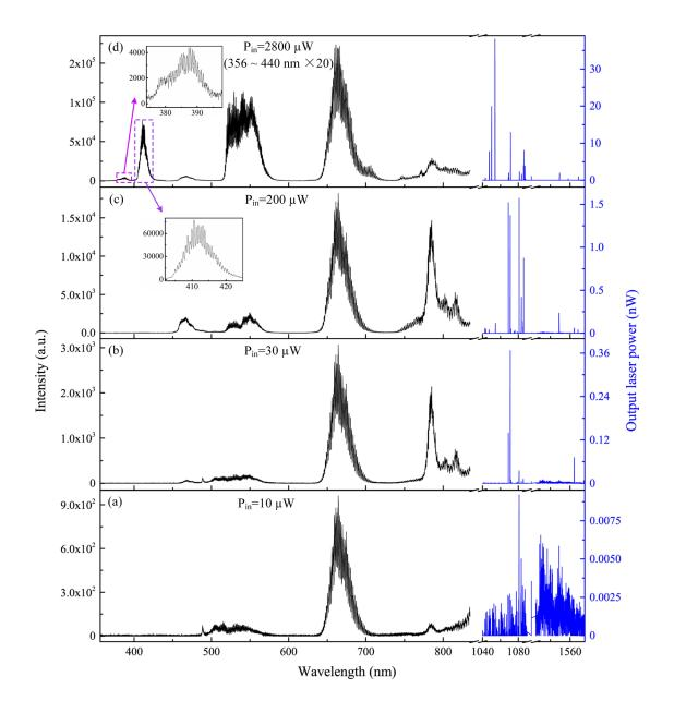
**Fig. S12.** Lasing spectrum evolution of MS1 with the increased pump power. The pump powers are (a) 10, (b) 30, (c) 200, (d) 2800  $\mu$ W, respectively, from the bottom to the top.
