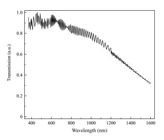
Fig. S7. Theoretical simulation of the transmission spectrum. The diameters of the microfiber and the microsphere are 1.2 and 57  $\mu$ m, respectively. The microfiber is glued to the equator of the microsphere.
