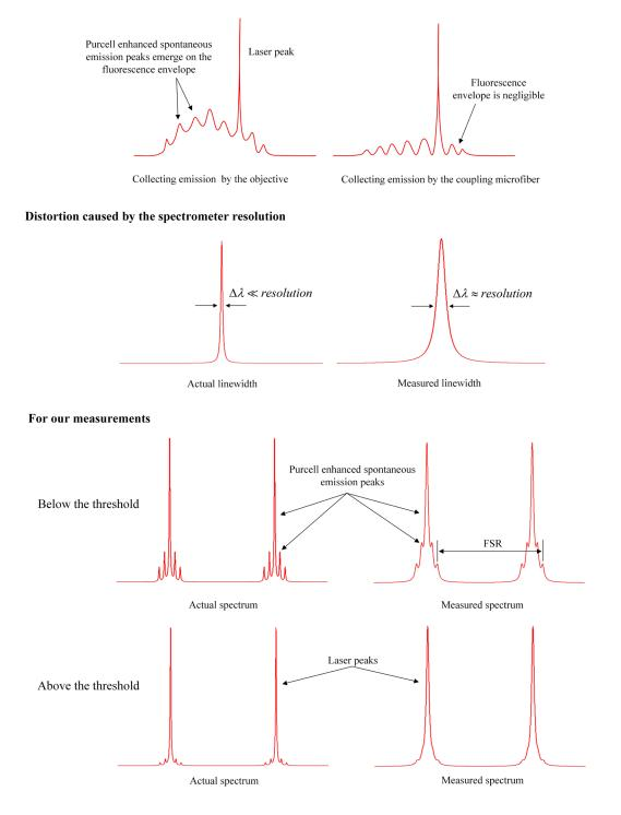
Fig. S8. Schematic of optical spectrum acquisition.
