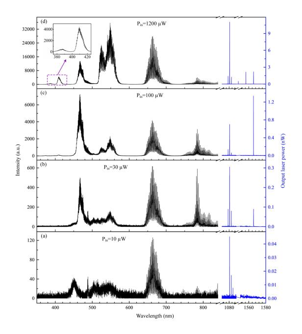
Fig. S14. Lasing spectrum evolution of MS2 with the increased pump power. The pump powers are (a) 10, (b) 30, (c) 100, (d) 1200  $\mu$ W, respectively, from the bottom to the top.
