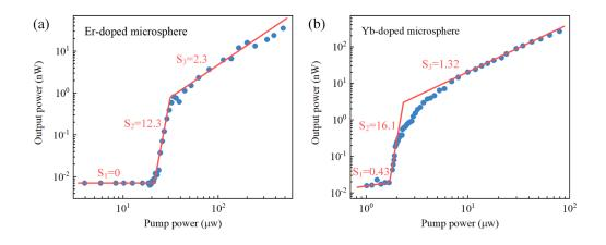
**Fig. S5.** Emission intensities in the (a) 1550 and (b) 1080 nm-bands versus the pump power in log-log scale, where S represents the slope.
