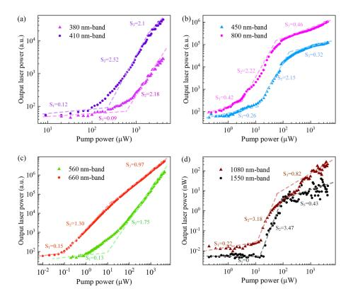
**Fig. S11.** Emission intensity of MS1 versus the pump power in log-log scale. The upconversion emission intensities are integrated from (a) 380 to 396 and 402 to 426 nm, (b) 450 to 489 and 756 to 816 nm, (c) 555 to 575 and 645 to 590 nm. (d) The downshifting emission intensities are summarized from the intensities of individual lasing wavelengths.
